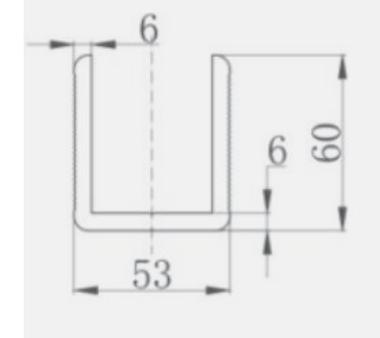
Technical drawing showing dimensions: 53 (width), 6 (flange thickness), 60 (height), and 6 (flange offset).
