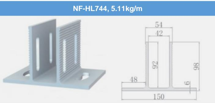
Technical drawing showing dimensions: 150 (width), 48 (base offset), 92 (height), 51 (top width), 42 (inner top width), 6 (flange thickness), and 98 (total height).
