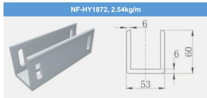
Technical drawing showing dimensions: 53 (width), 6 (flange thickness), 60 (height), and 6 (flange offset).
